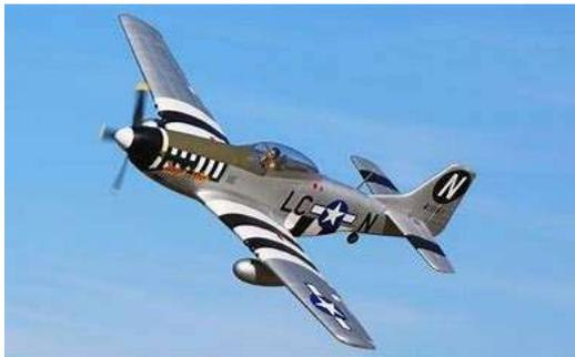
The plane that gave the American Airforce air superiority over the Luftwaffe was the North American Mustang. It combined American design, the Rolls Royce Merlin, lamina flow wing and the work of a British scientist on the engine cooling system.
