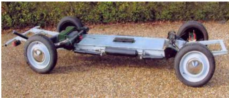
The new galvanised steel chassis arrived (See Pic) and it shows the start of the rebuild. Many people think that the 2CV has torsion bar suspension but the picture shows the actual arrangement. The car has independent suspension with rods coming from the
