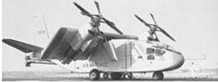
The X-18 with partially rotated wings
