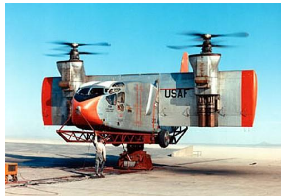
The X-18 on its test stand
